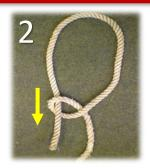
Pass the short free end of the rope through the small loop.
